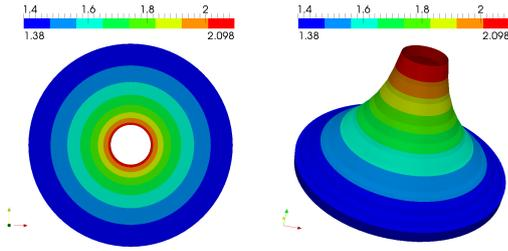
Figure 4: Temperature plot (FVM)
